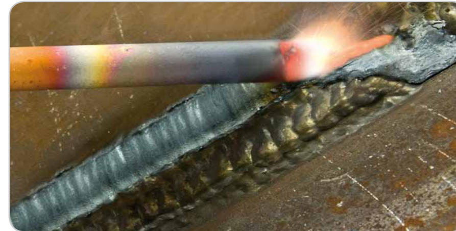
KempGouge ARC 800 makes easy work of carbon arc gouging tasks.
