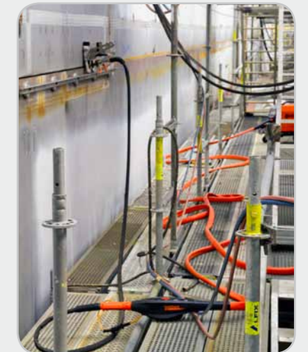
MagTrac F 61 is fully compatible with Kemppi's SuperSnake subfeeder, which gives you up to 15 meters of further reach.
