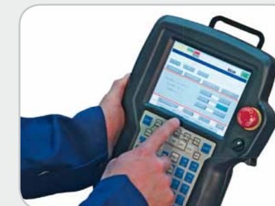
Robot control pendant displaying KempArc Browser interface.
